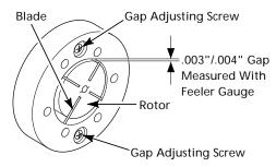
Figure 19 - Gap Adjusting Screw Locations
